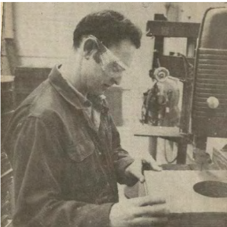
Jerry Manus custom cuts cardboard on the band saw and shapes it to fit customer specifications.
